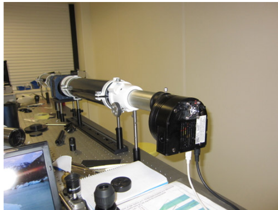
Fig. 8. Optical system compound by the two telescopes used for obtaining a measure of the resolution.
