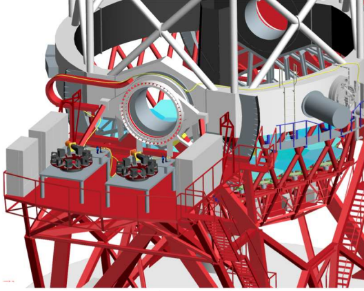
Fig. 1. 3D model of MEGARA at the 10.4 m GTC. All, the Folded-Cass subsystem, the fiber routing and the MEGARA spectrograph at the Nasmyth platform are shown. Note that the expected final destination of the spectrograph according to the long-term instrumentation plans of GRANTECAN is a sub-Nasmyth platform.
