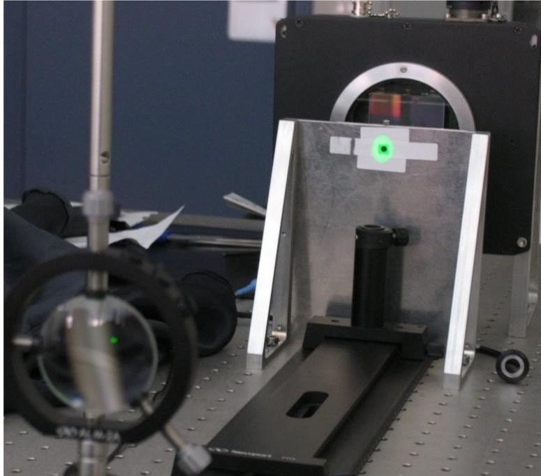
Figure 4. A CCD camera having its QE measured. The monochromator output can be seen focused onto a 5mm aperture placed just in front of the camera. The unused photodiode is visible on the optical bench at the right.
